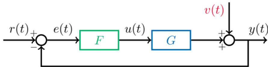
It is also important to study how disturbances affect the system. For example, with the disturbance  $v(t)$  as in the block diagram, we get
