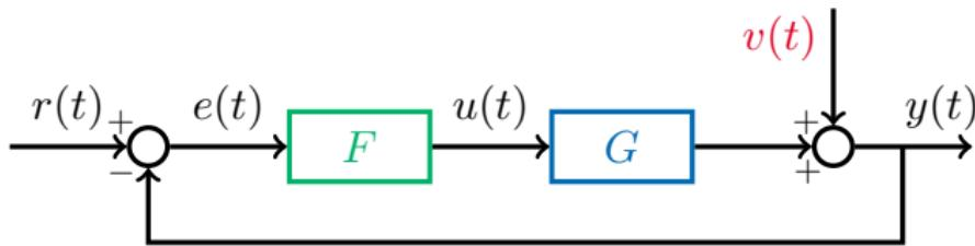
It is also important to study how disturbances affect the system. For example, with the disturbance  $v(t)$  as in the block diagram, we get
